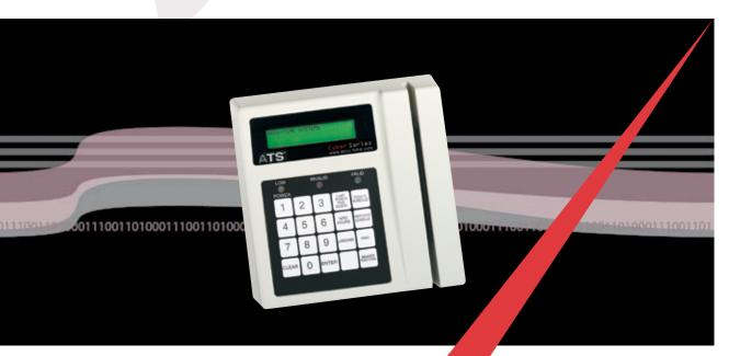
The Accu-Time Cyber Series is ideal for workforce management applications such as employee time and attendance for payroll, access control, and job tracking. This cost-effective Cyber terminal is a programmable data collection device with features previously reserved for the most expensive platforms. The selectable serial or Ethernet (10/100BASE-T) communications and ATS's Universal Command Set programming interface offer countless configuration options that make the Cyber Series second to none.
